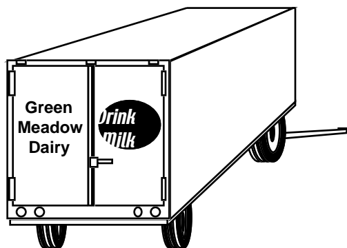
Figure 3. Van body on running gear for storing bagged materials.
