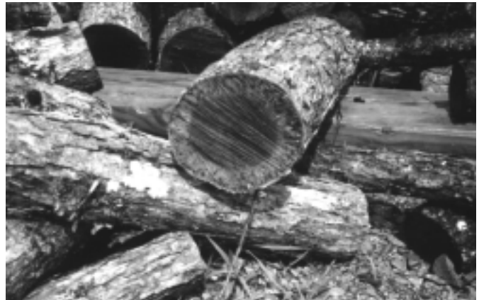
Figure 2. The lighter, outermost wood is the sapwood and the darker, inner wood is the heartwood.
