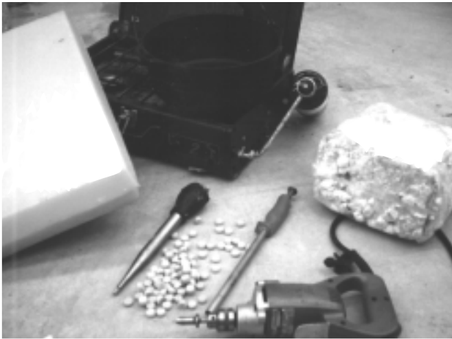
Figure 3. Equipment and supplies used for inoculation of logs. From left to right: cheese wax, propane stove, wax pot, wax baster (front), foam plugs (front), propane canister (rear), inoculation tool (front) spawn (rear), high speed drill, \frac{7}{16} inch bit with collar stop and screw tip.
