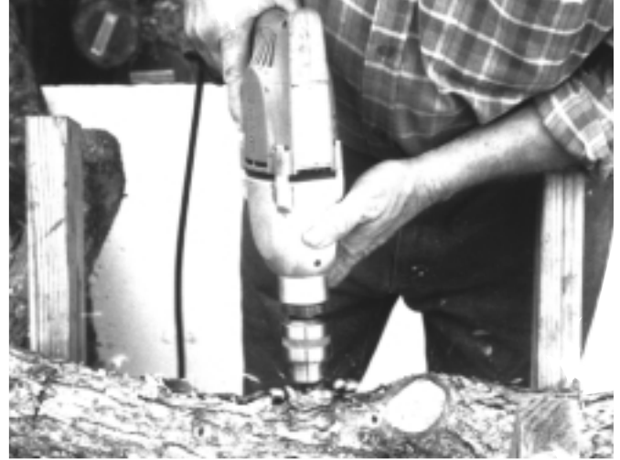
Figure 4. Drill down the length of the log.
